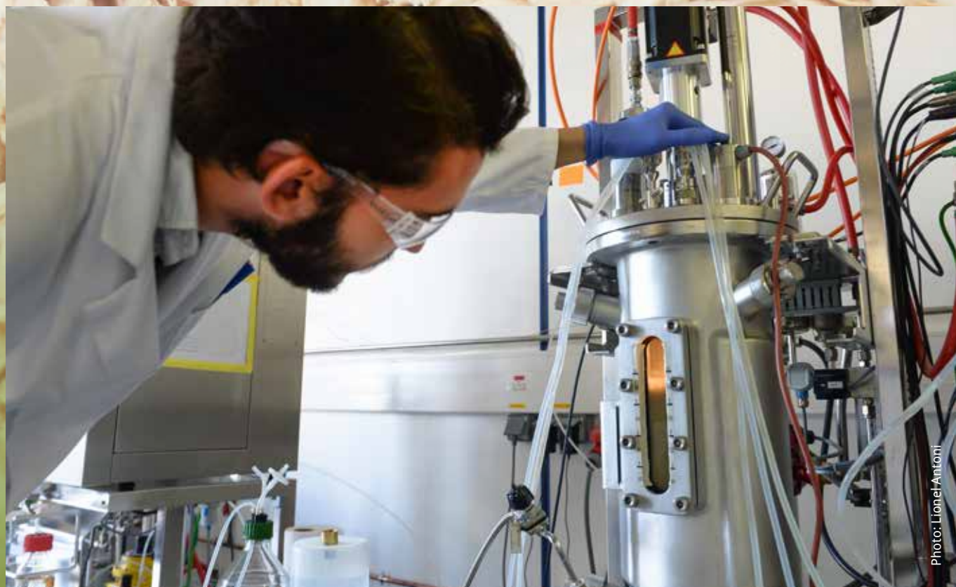
At this demonstration plant, Global Bioenergies produces high purity isobutene at ton scale, which will be converted into plastics, fuels, rubber or cosmetic ingredients.
